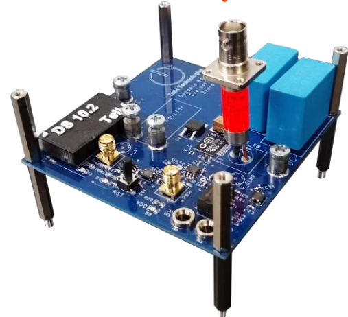
Dynamic R_{DS-ON} Evaluation Board #Tell-i-Eval-DynR-B
