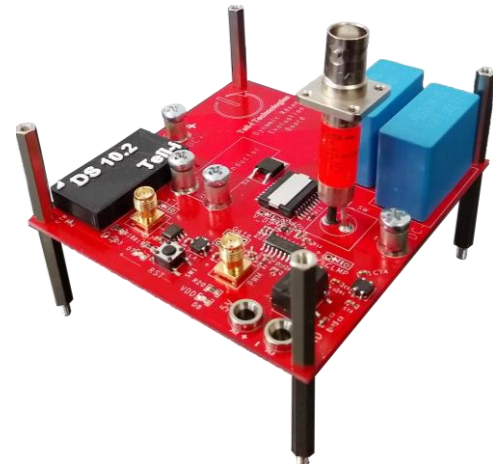
Dynamic R_{DS-ON} Evaluation Board #Tell-i-Eval-DynR-A
