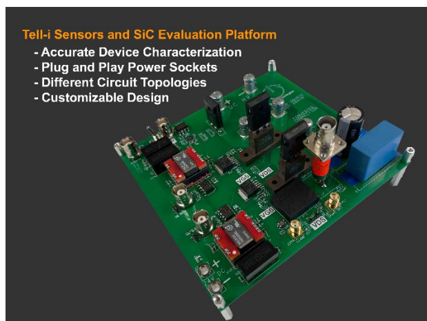
Figure 4. Samples of system design kits to evaluate different WBG (SiC and GaN) devices and Tell-i sensors.
